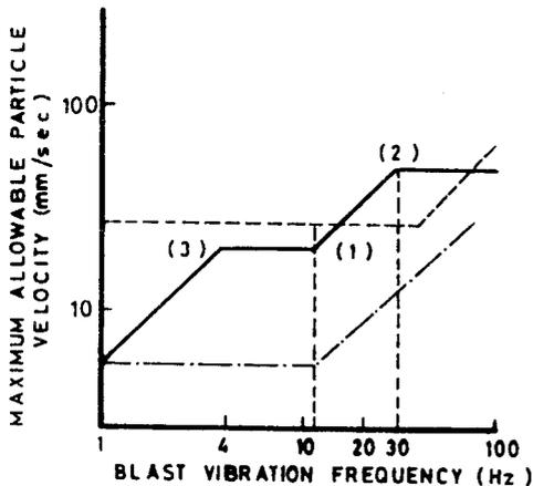
NOTE — Dotted line has been employed safely for close construction blasting near engineered structures. Dashed line has been employed safely for construction blasting in urban areas near older homes and historic buildings.
