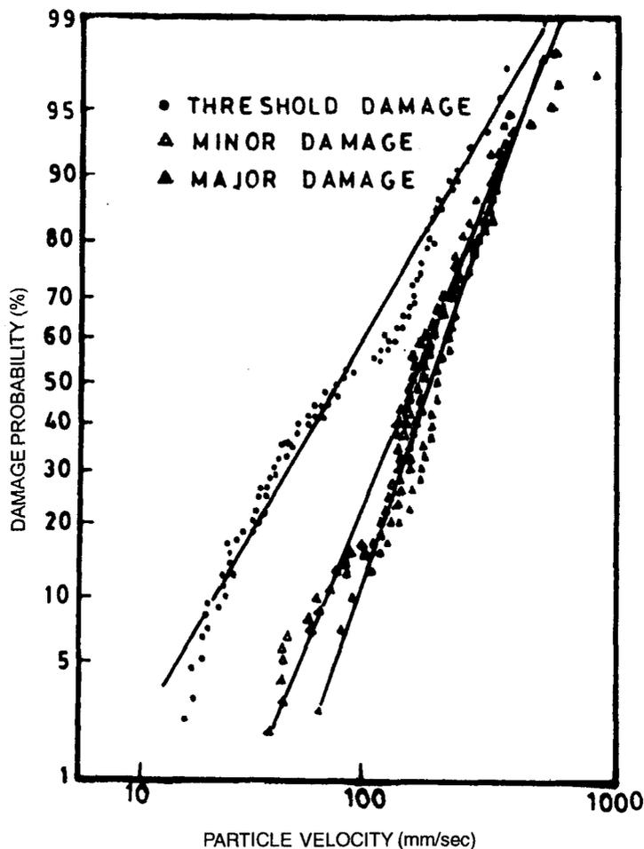
FIG. 7 PROBABILITY ANALYSIS OF BLAST CRACKING DATA
