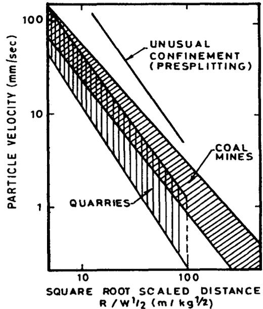
FIG. 3 ATTENUATION RELATIONSHIPS SHOWING SCATTER FROM GEOLOGICAL AND BLAST DESIGN EFFECTS AS WELL AS HIGH EXPECTED VELOCITIES FROM CONFINED SHOTS, SUCH AS PRE-SPLITTING
