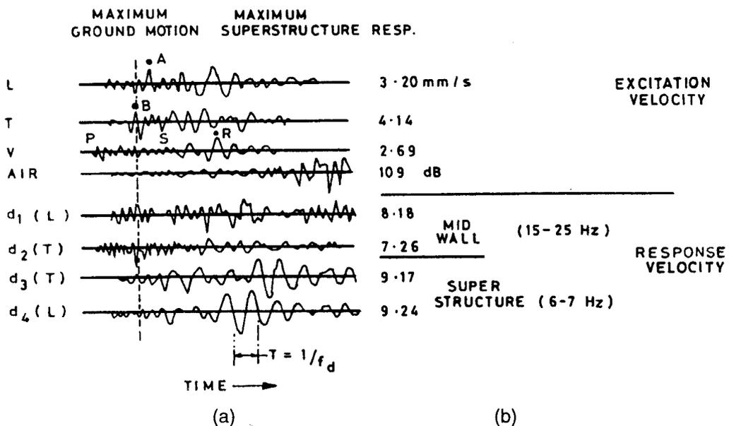
FIG. 1 COMPARISON OF (a) BLAST EXCITATION BY GROUND AND AIR-BORNE DISTURBANCES AND (b) RESIDENTIAL STRUCTURE RESPONSE OF WALLS AND SUPERSTRUCTURE
