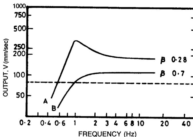
FIG. 6 TYPICAL RESPONSE SPECTRA OF A VELOCITY TRANSDUCER WITH DIFFERING PERCENTAGES OF DAMPING WITH 70 PERCENT OF CRITICAL DAMPING
