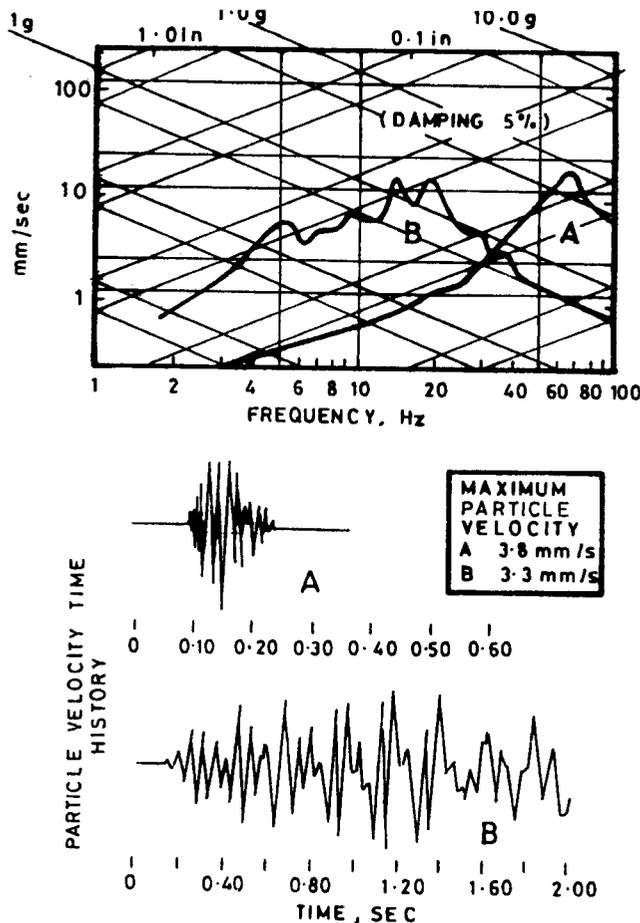
FIG. 8 COMPARISON OF TIME HISTORIES SPECTRA FROM CONSTRUCTION AND SURFACE MINING BLASTS RESPECTIVELY LASTING 0.15 AND 2.0 SECONDS
