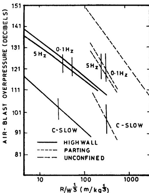
FIG. 4 ATTENUATION RELATIONSHIPS FOR AIR OVER-PRESSURES PRODUCED BY CONFINED (HIGH WALL) AND PARTIALLY CONFINED (PARTING) SURFACE COAL-MINING BLASTS AS WELL AS UNCONFINED BLASTS
