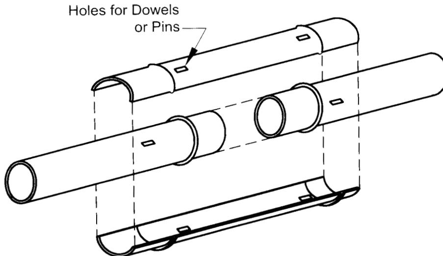
FIG. 3 BUTT JOINT WITH SIDE PLATES IN BAMBOO
