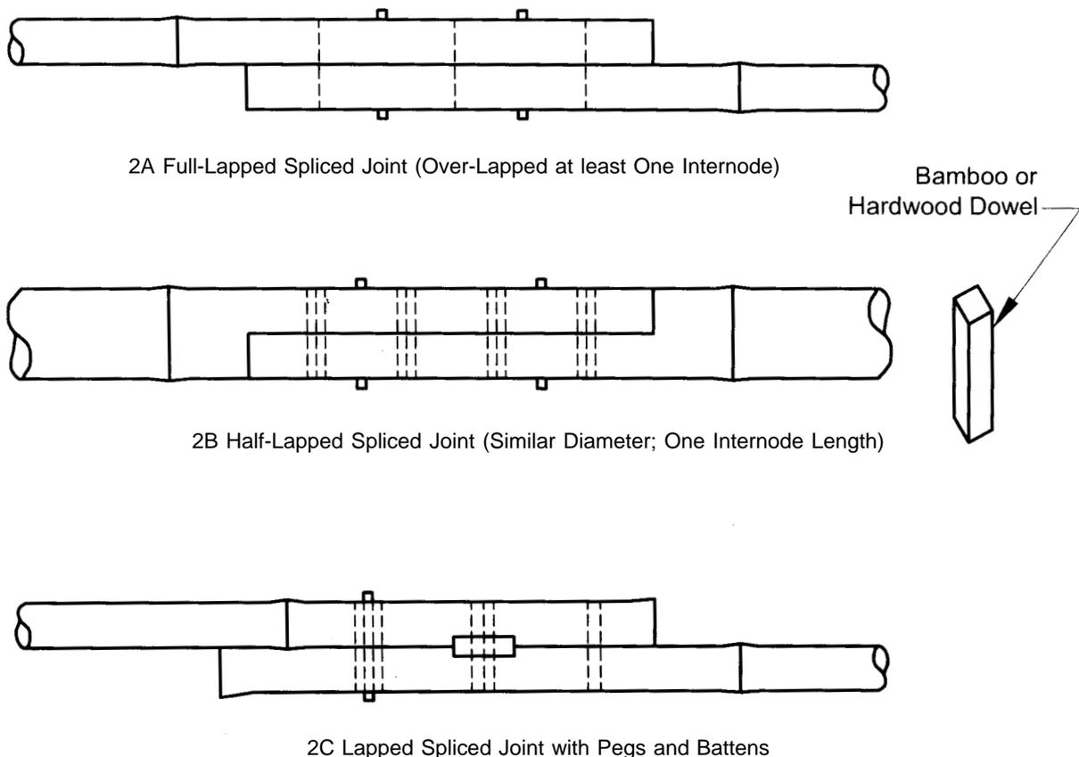
FIG. 2 LAP JOINTS IN BAMBOO
