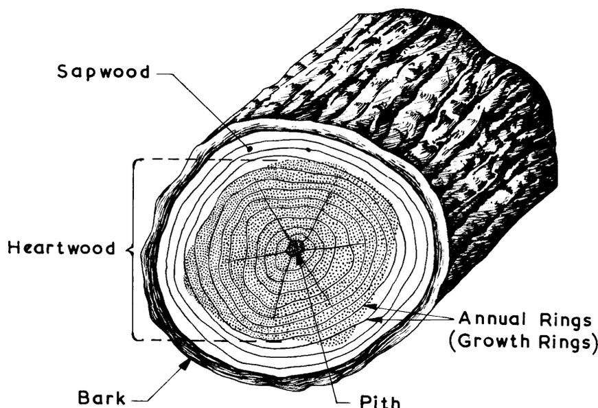
FIG. 1 CROSS-SECTION OF LOG
