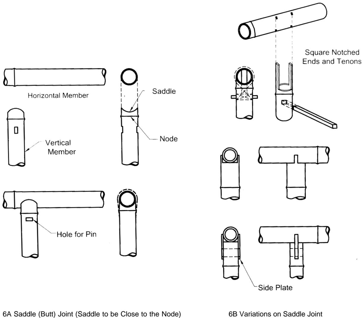
FIG. 6 BUTT JOINTS IN BAMBOO
