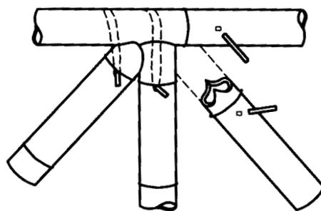
FIG. 9 ANGLED JOINT IN BAMBOO WITH INTEGRAL TENONS
