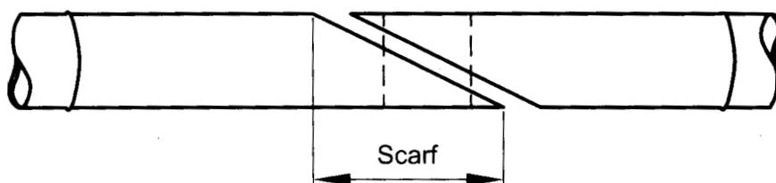
FIG. 5 SCARF JOINT IN BAMBOO
