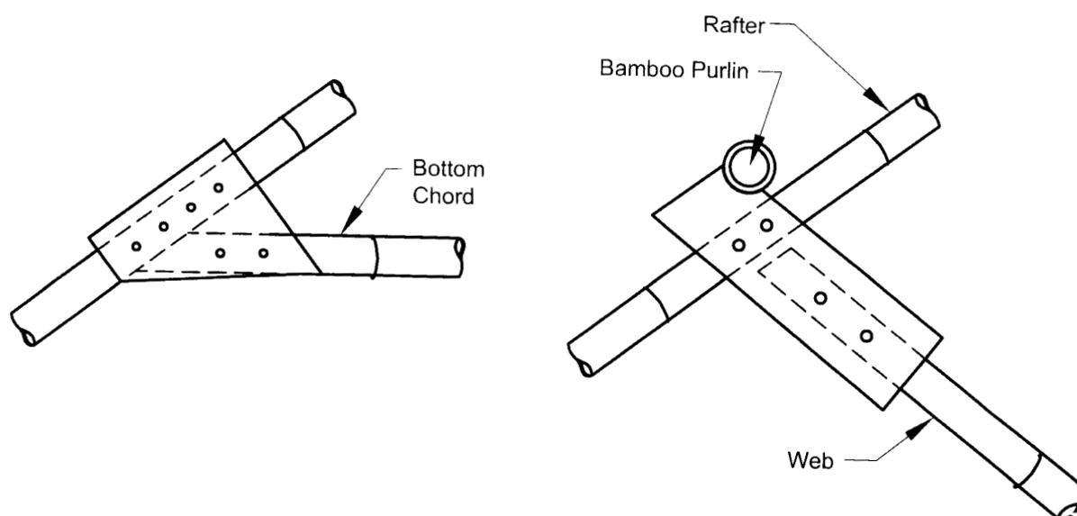
FIG. 10 GUSSET PLATED JOINTS IN BAMBOO
