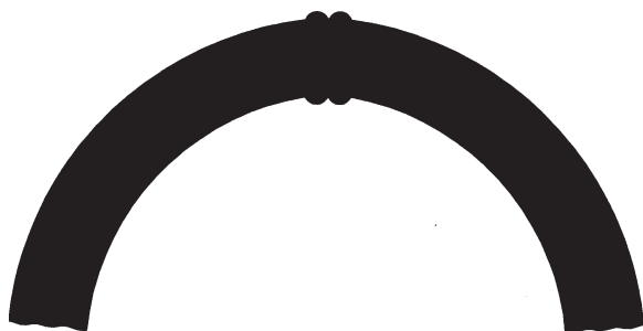
FIG. 3 BEND STRAP TEST — WELDED PIPE PORTION CUT LONGITUDINALLY AND BENT
